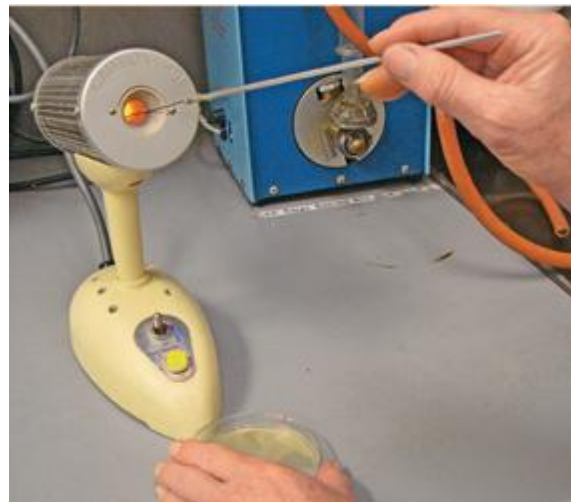
Figure B – Dry heat incineration using an infrared incinerator
