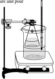
4) Remove the flask from the water bath by loosening the clamp from the supporting rod and moving it upward. Allow the flask to cool to room temperature, and dry it on the outside gently and thoroughly with a paper towel. Weigh the flask along with its contents, the aluminum foil and rubber band, and record this value on the report form.
