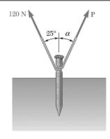
For the stake of Prob. 2.5, knowing that the tension in one rope is 120 N, determine by trigonometry the magnitude and direction of the force  $\bf P$  so that the resultant is a vertical force of 160 N.
