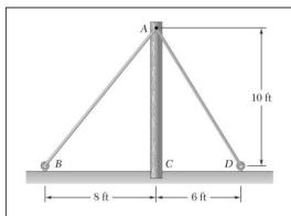
The cable stays AB and AD help support pole AC. Knowing that the tension is 120 lb in AB and 40 lb in AD, determine graphically the magnitude and direction of the resultant of the forces exerted by the stays at A using (a) the parallelogram law, (b) the triangle rule.
