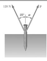
A stake is being pulled out of the ground by means of two ropes as shown. Knowing that  $\alpha = 30^{\circ}$ , determine by trigonometry (a) the magnitude of the force **P** so that the resultant force exerted on the stake is vertical, (b) the corresponding magnitude of the resultant.
