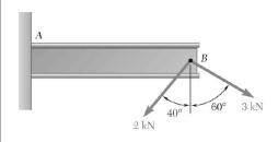
Two forces are applied at point B of beam AB. Determine graphically the magnitude and direction of their resultant using (a) the parallelogram law, (b) the triangle rule.
