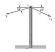
A telephone cable is clamped at A to the pole AB. Knowing that the tension in the right-hand portion of the cable is  $T_2 = 1000$  lb, determine by trigonometry (a) the required tension  $T_1$  in the left-hand portion if the resultant  $\mathbf{R}$  of the forces exerted by the cable at A is to be vertical, (b) the corresponding magnitude of  $\mathbf{R}$ .
