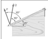
Two forces **P** and **Q** are applied to the lid of a storage bin as shown. Knowing that P = 60 N and Q = 48 N, determine by trigonometry the magnitude and direction of the resultant of the two forces.
