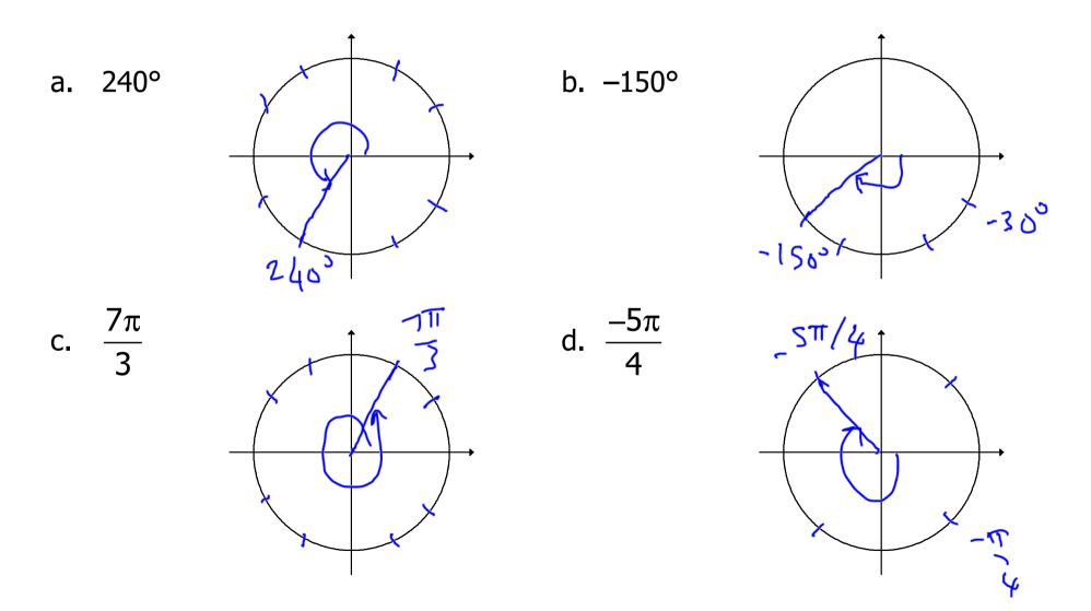
Angles that have the same terminal side are called co-terminal angles. Measures of co-terminal angles differ by a multiple of 360° if measured in degrees or by multiple of  $2\pi$  if measured in radians.
