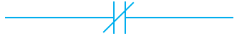
Figure 5.16 Symbol for a normally closed pole of a relay or contactor. (Delmar/Cengage Learning)
