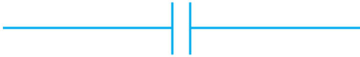
Figure 5.15 Symbol for a normally open pole of a relay or contactor. (Delmar/Cengage Learning)
