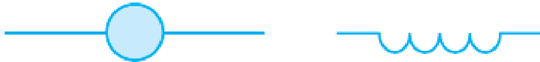
Figure 5.17 Symbols for relay or contactor coil; either symbol may be used for each device. (Delmar/Cengage Learning)
