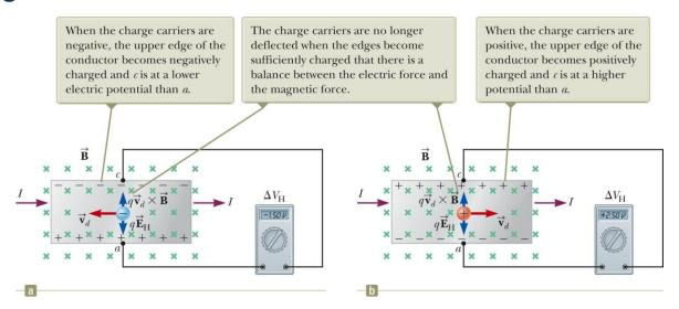
When the charge carriers are negative, they experience an upward magnetic force, they are deflected upward, an excess of positive charge is left at the lower edge.
