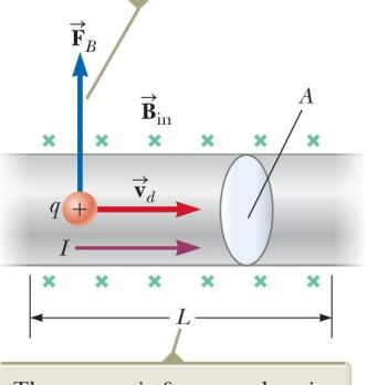
The magnetic force on the wire segment of length L is  $I\vec{L} \times \vec{B}$ .
