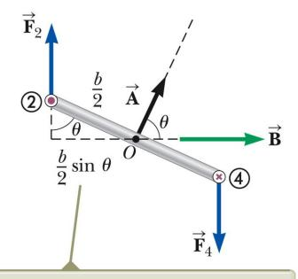
When the normal to the loop makes an angle  $\theta$  with the magnetic field, the moment arm for the torque is  $(b/2) \sin \theta$ .
