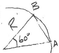
$$\text{P-wave dist} = 2R \sin 30^\circ = 2(6.37 \times 10^6 \text{ m}) \sin 30^\circ = 6.37 \times 10^6 \text{ m}$$
